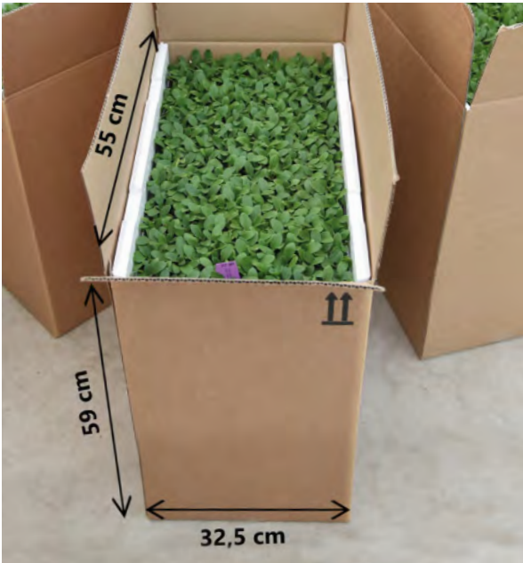
Box dimensions for five trays of trailing petunia young plants stacked in "high" polystyrene tray-holders and subsequently placed in cardboard boxes, ready for despatch.
